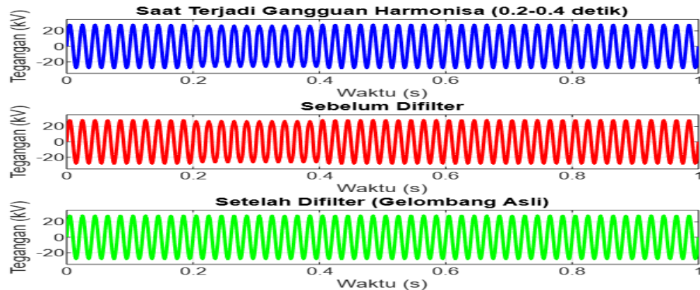
Figure 4. Simulation results of normal signals, with harmonics and after filtering.
