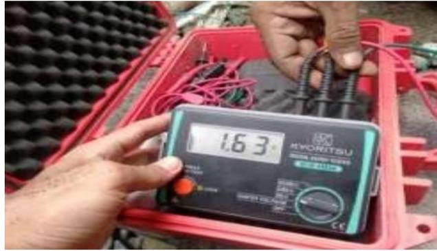
**Gambar 3.** Pengukuran Tahanan Sistem Pentanahan Bak Kontrol Grounding
