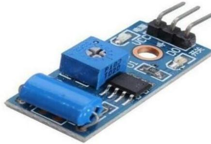
Gambar 1. Sensor Getaran (Vibration)
